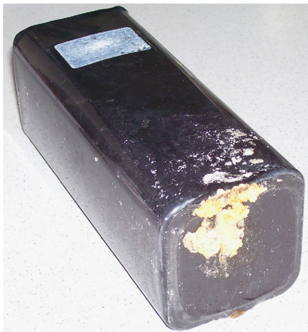
Fig. 1. Salt deposits U on the case of a burst ultracapacitor after extended operation at high temperatures and abusive voltages.
